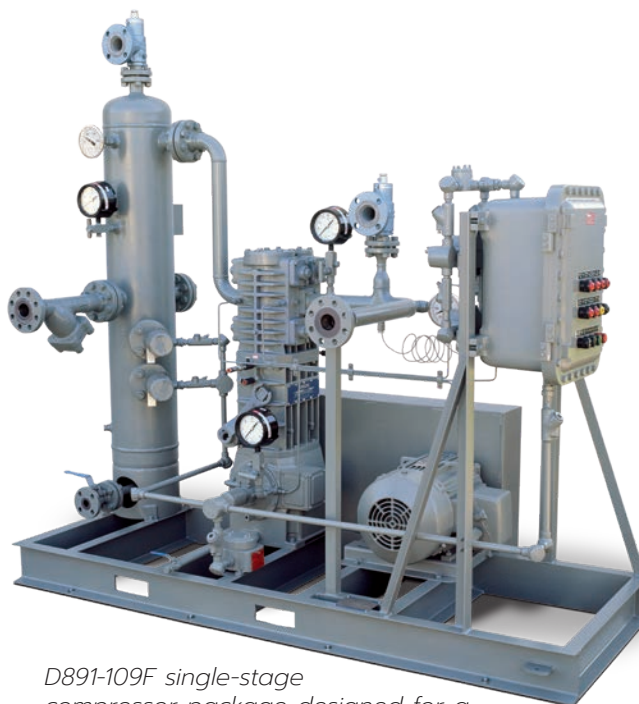
Customized D891-109F single-stage compressor package designed for a liquefied gas transfer application.
