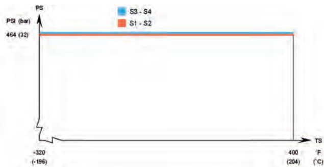
CB400 - UL approval pressure/temperature graph*
