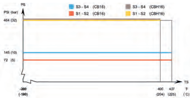
CB16 / CBH16 - CRN approval pressure/temperature graph
